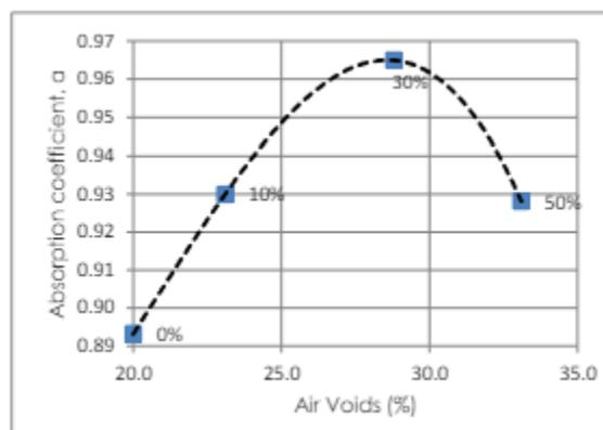
**Figure 1.11 Correlation between sound absorption vs. air voids**
