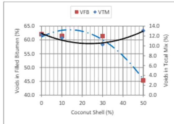
**Figure 1.7 Relationship between VFB and VTM at different percentage coconut shell**
