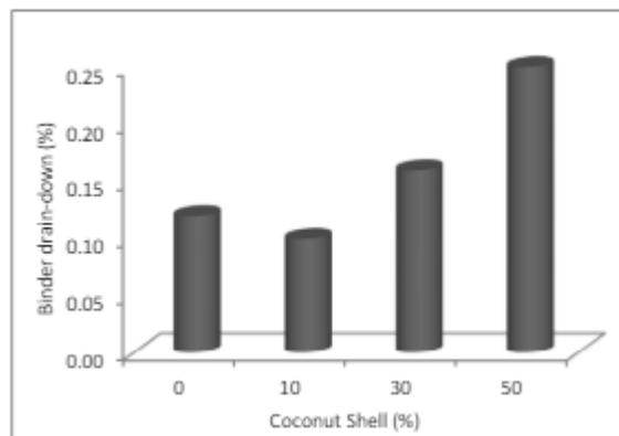
**Figure 1.9 Binder drain-down of porous asphalt mixture incorporating coconut shell**
