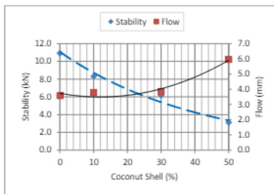
**Figure 1.6 Relationship between stability and flow at different percentage coconut shell**
