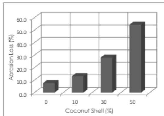
**Figure 1.8 Loss of abrasion porous asphalt mixture incorporating coconut shell**
