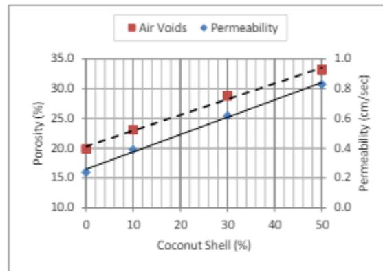
**Figure 1.12 Correlation between porosity and permeability at different level coconut shell**
