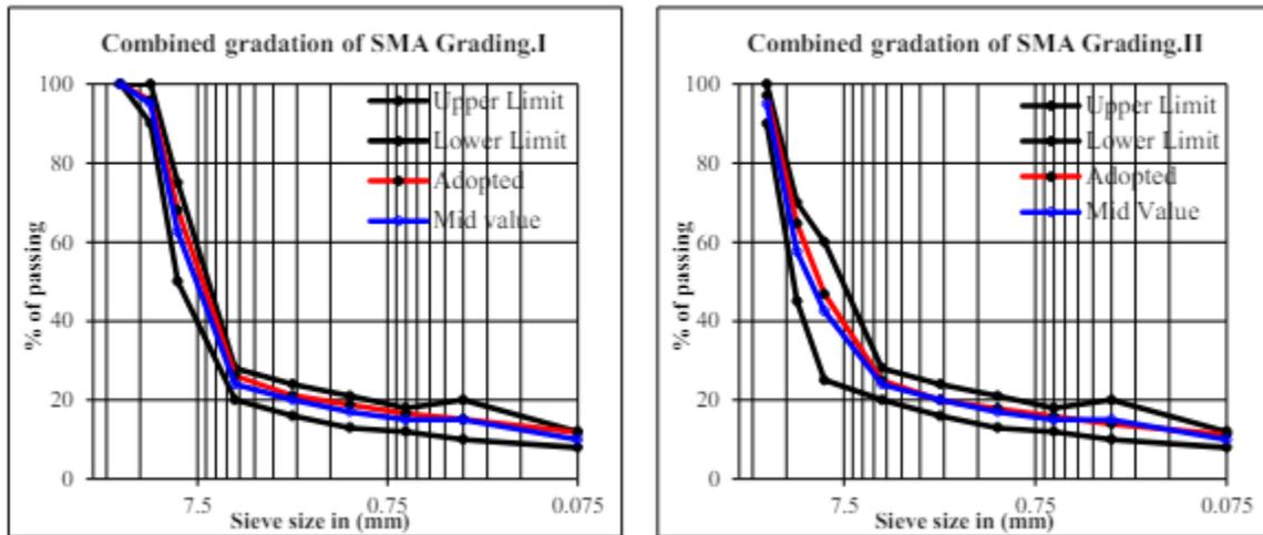
**Figure 1.1 Gradation curve of SMA using IRC: SP: 79-2008 Figure 4 Gradation curve of SMA using IRC: SP: 79-2008**
