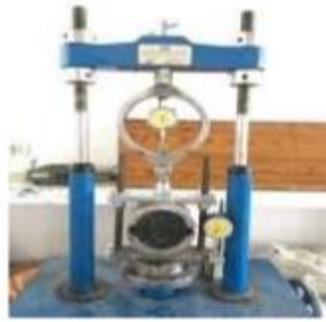
**Figure 1.3 Marshall stability testing machine**
