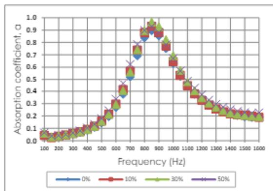
**Figure 1.10 Sound absorption coefficients at varying coconut shell replacement**
